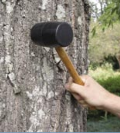
Sounding for decays and hollows
